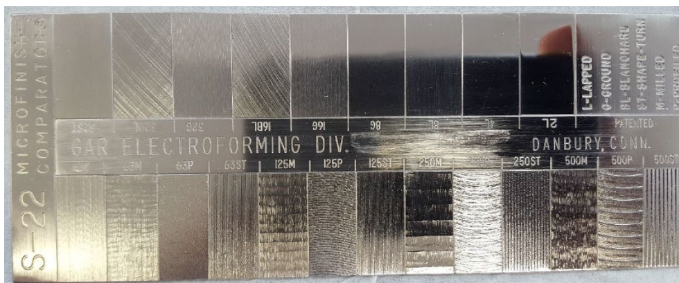
Figure 1. Surface finish comparator used for gauging effects of surface roughness on contact angle measurements. This device consists of nickel-plated steel.
