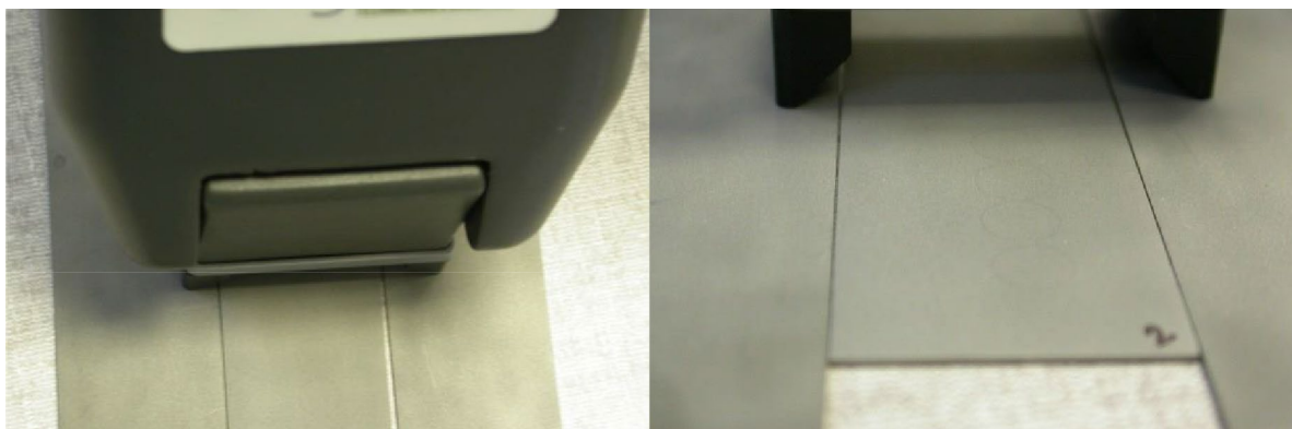
Figure 3. Images illustrating how two additional coupons were used to control the spacing between the Surface Analyst and the coupon to be measured.
