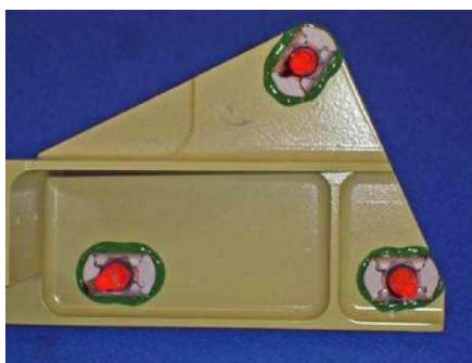
Figure 3: Nutplates bonded to an aluminum casting. Orange elastomer tabs passing through threaded fastener are for fixturing during adhesive cure and are removed prior to use.
