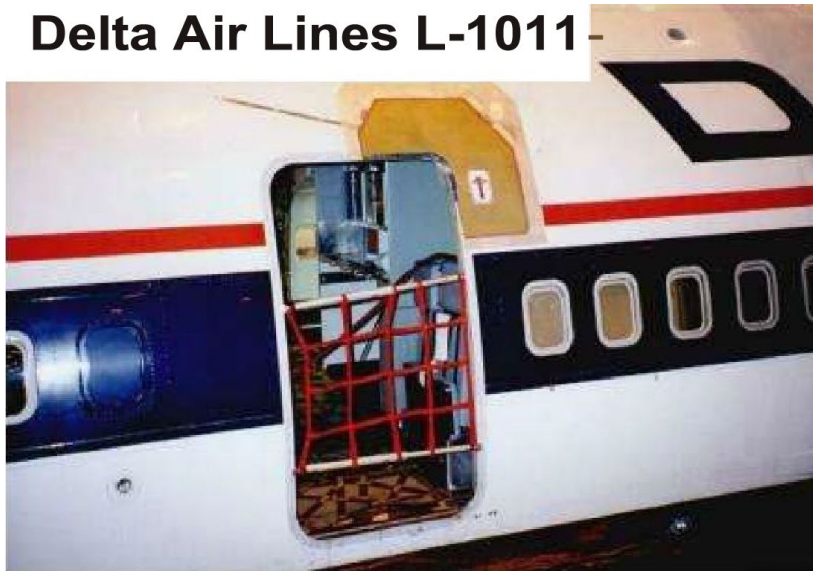
Figure 1: Bonded boron/epoxy composite doubler for repair of aluminum aircraft [1].
