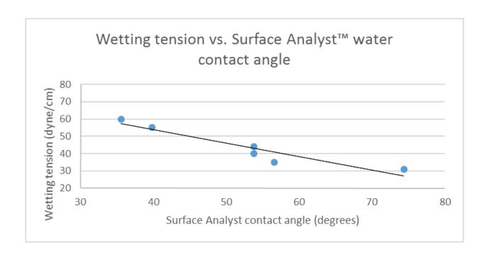
In the range of dyne test inks used in this evaluation—30-60 mN/m—the relationship between wetting tension and contact angle is quite linear. This relationship allows BTG Labs to provide the option of dyne readout on the SA3001. Customers who are accustomed to dyne readings can easily have the option of continuing to utilize that scale.
