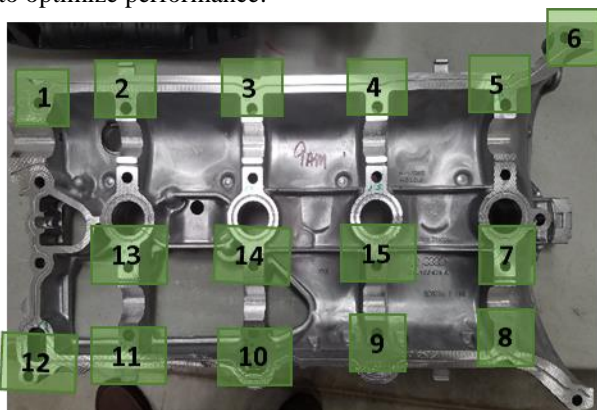
Figure 2. Inspection points on machined engine sealing surfaces evaluated for cleanliness via Ballistic water contact angle measurements.
