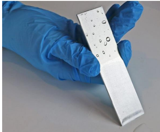
Figure 1. Depiction of water break test results. Top portion of the panel displays a non-water break free surface (water beads up). Bottom portion displays a water break free surface (water spreads out).
