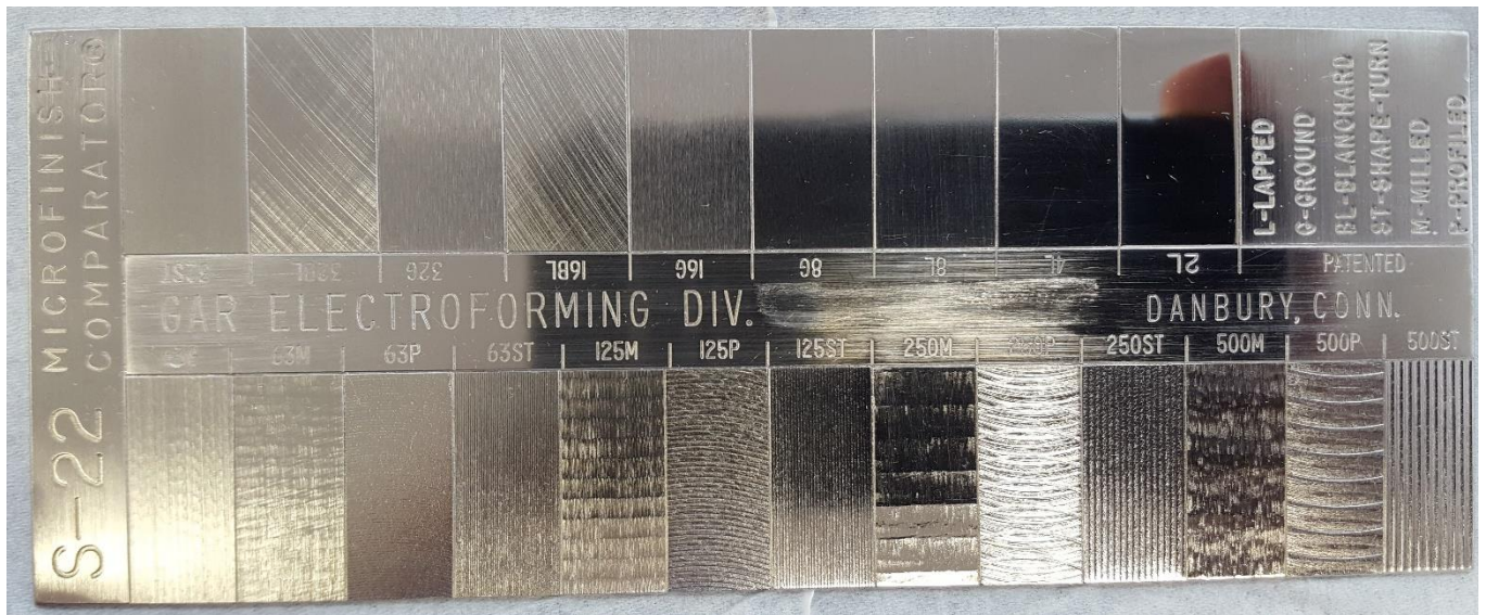
Figure 1. Surface finish comparator used for gauging effects of surface roughness on contact angle measurements. This device consists of nickel plated steel.
