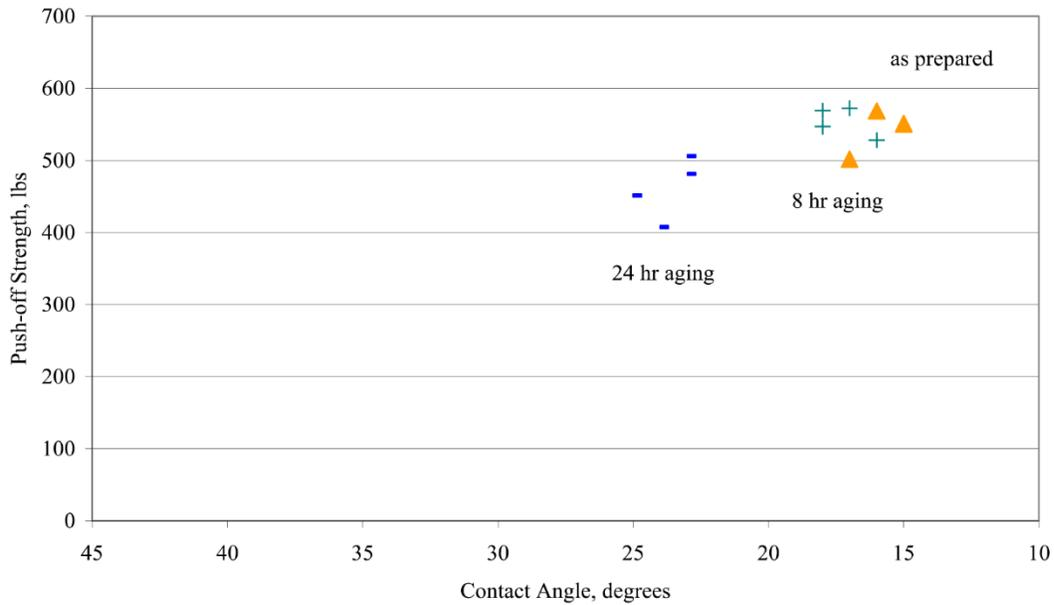
Figure 8. Push off load vs. contact angle for abraded and aged graphite/epoxy substrates.
