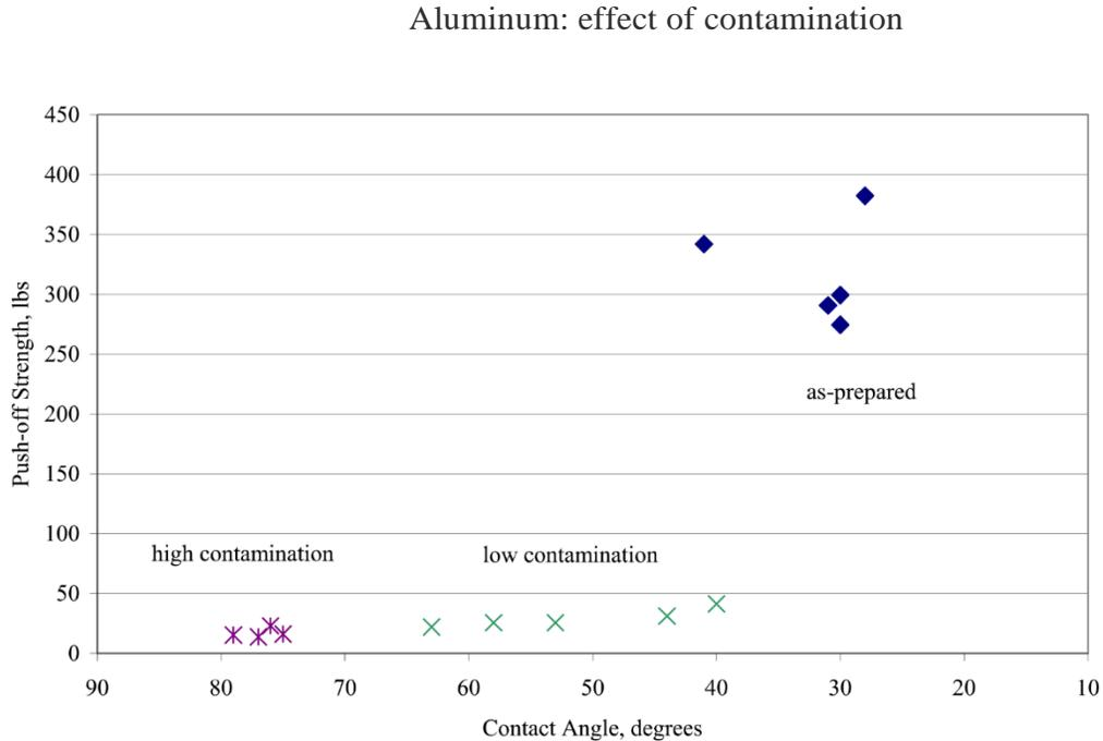
**Figure 9.** Push off load vs contact angle for abraded and contaminated Al substrates.
