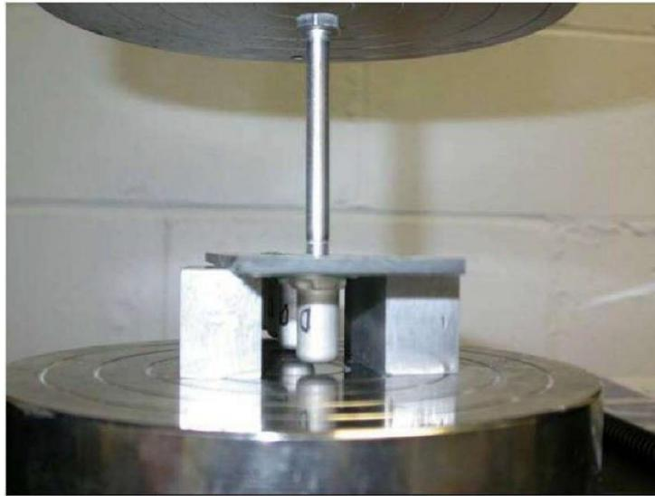
**Figure 4.** Determination of bond strength of nutplates.
