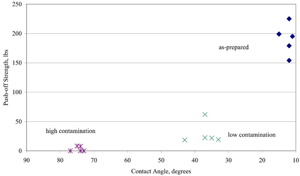
**Figure 10.** Push off load vs. contact angle for abraded and contaminated Ti-6Al, 4V substrates.
