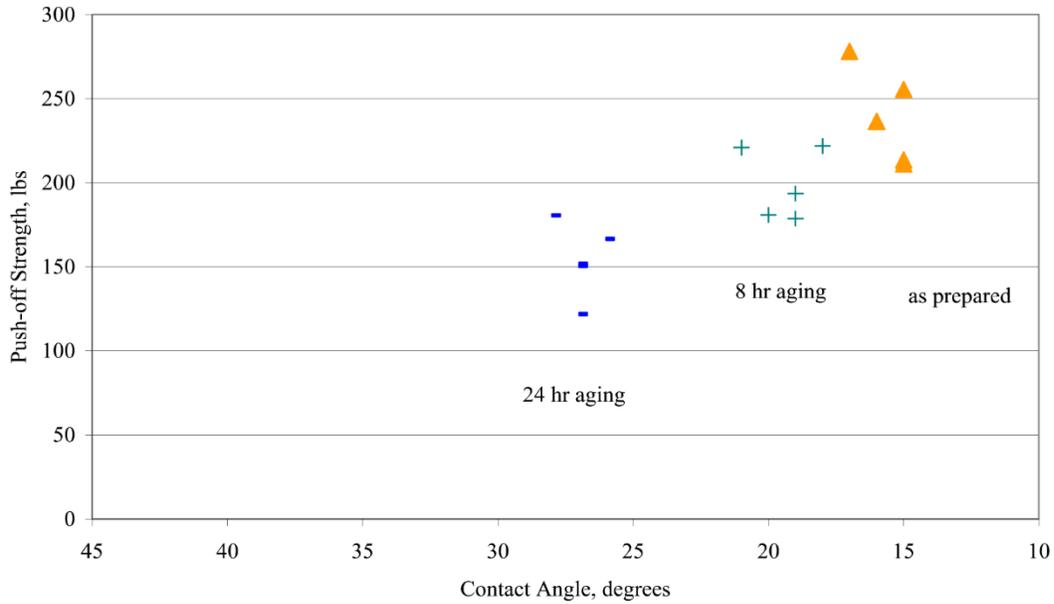
Figure 7. Push off load vs. contact angle for abraded and aged Ti-6Al, 4V substrates.
