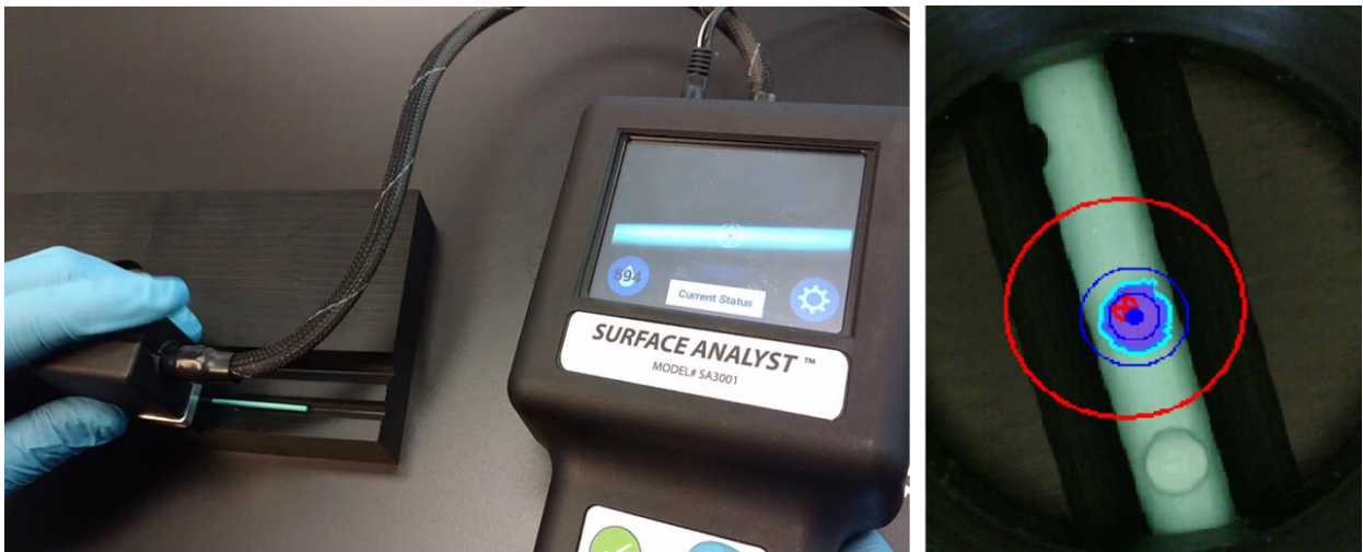
Figure 6. Left: Surface Analyst SA3001 contact angle instrument. 6Fr tubing sample can be seen in the black fixture. Right: example of automated drop shape analysis on Ballistically Deposited 0.6µl water drop.
