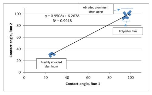
The next Figure shows the results obtained using the Surface Analyst on these same three surfaces. Contact angles on the polymer film and aged aluminum were lower than for the syringe deposited drops, as these surfaces show hysteresis and have a lower receding contact angle. The repeatability was excellent (R<sup>2</sup>=0.99). Most importantly, the data shows three clearly distinct populations of contact
