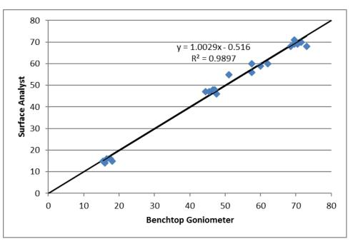
The correlation is excellent (R<sup>2</sup>=0.99), the slope is indistinguishable from 1.00, and there is less than 1° offset, confirming the validity of the top-down measurement system used in the Surface Analyst.
